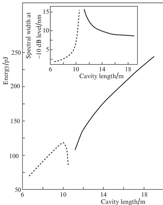
**Figure 4.** Output pulse energy and the spectral width vs. the cavity length. The dashed curves correspond to the regimes with normal average dispersion, the solid curves to those with anomalous dispersion.
