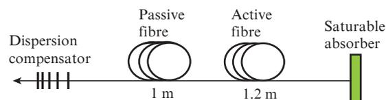
**Figure 1.** Scheme of a fibre laser.
