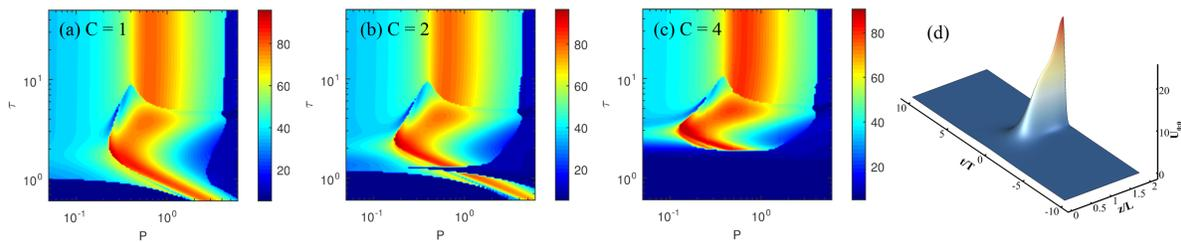
Fig. 2. The dependence of the percentage of total energy  $E$  combined in the central core at the first local maximum of the peak power of input pulse on the parameters  $P$  and  $\tau$  of input Gaussian pulses for the hexagonal 19-core MCF with various values of chirp parameter  $C$ . Dynamic of the field in the center core for the best combining case ( $C = 2, P = 1.776, \tau = 2.34$ ) with 96.5% of energy combining.
