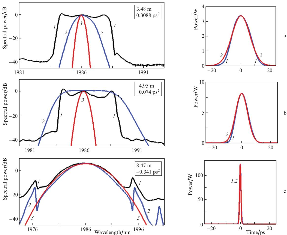
**Figure 3.** Comparison of the spectra obtained in the experiment (1), using the numerical method (2), and the Gaussian spectrum reconstructed from the characteristics of the calculated pulse (3) (left); comparison of the calculated pulse shape (1) with that of the reconstructed Gaussian pulse (2) (right).
